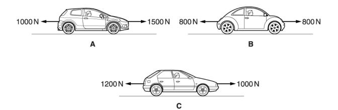
Put a tick  $(\checkmark)$  in the correct box in the table below to show if each car is moving at a steady speed, increasing speed or decreasing speed.
