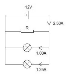
Calculate the power dissipated by resistor R.
