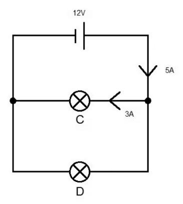
Use the formula resistance = potential difference ÷ current to calculate the resistance of bulb D.
